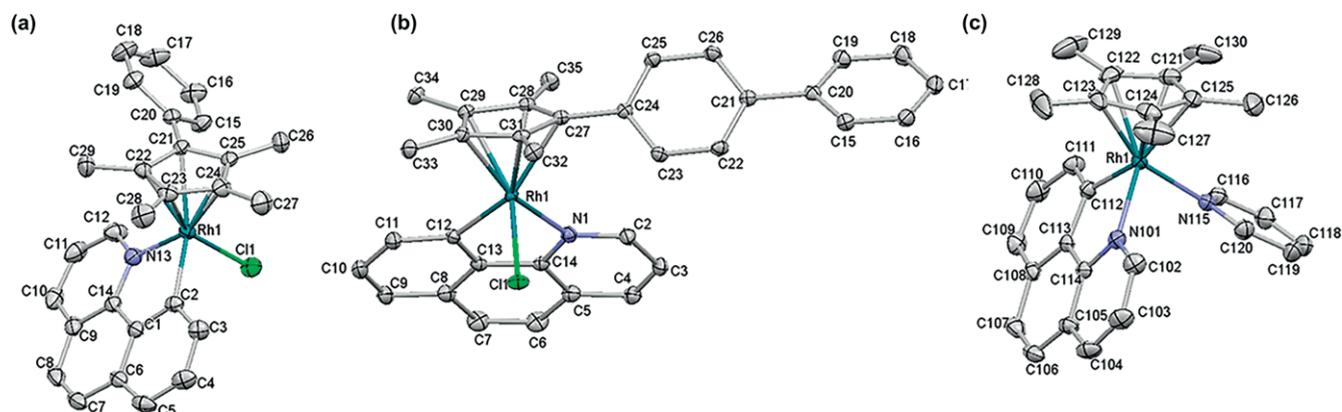
Figure 1. X-ray structures with atom numbering of (a)  $[\text{Cp}^{\text{Ph}}\text{Rh}(\text{benzo}[h]\text{quinoline})\text{Cl}]$  (**2a**); (b)  $[\text{Cp}^{\text{biph}}\text{Rh}(\text{benzo}[h]\text{quinoline})\text{Cl}]$  (**3a**); (c)  $[\text{Cp}^{\text{Ph}}\text{Rh}(\text{benzo}[h]\text{quinoline})\text{pyridine}]\text{PF}_6$  (**1b-PF<sub>6</sub>**), drawn with thermal ellipsoids at 50 % probability. Hydrogen atoms and counterions have been omitted for clarity.
