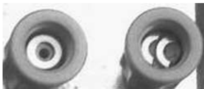
Figure 11 Catheter assembly (opened up) showing Left: normal disc and central lumen of the rubber cylinder; Right: two pieces of the disc; one overlying the central lumen of the rubber cylinder.
