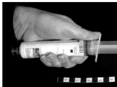
Figure 8 Moderate force is required to disengage the plastic flange from the glass syringe.
