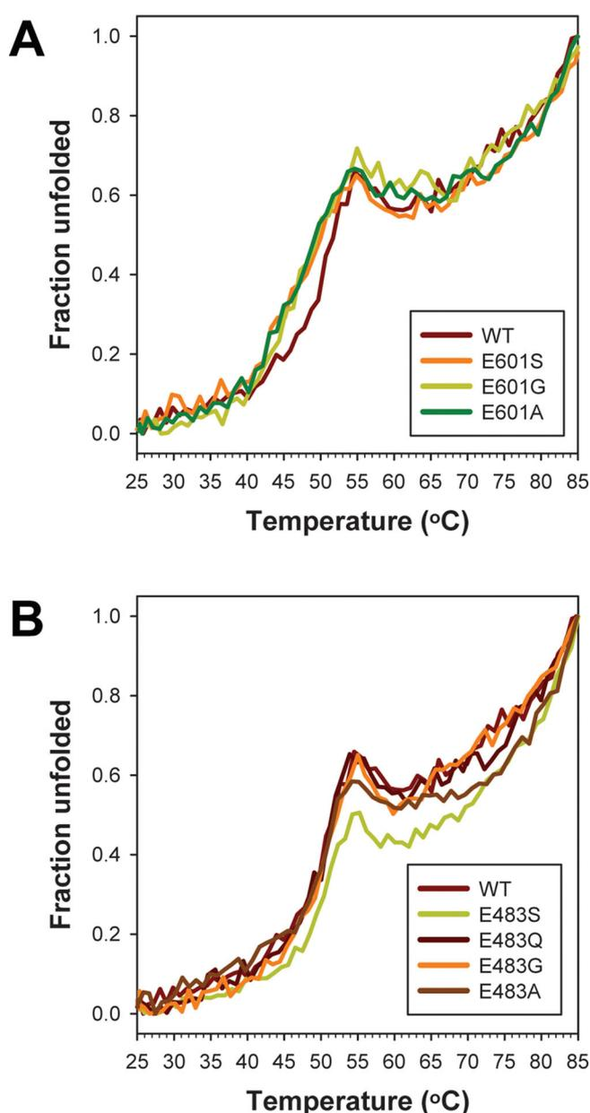
**Figure 2.** *CpGH89* structure-based stability. **A:** Melting curves of *CpGH89* and its Glu601 mutants measured by following the change in CD absorption at 220 nm by heating from 25 °C to 85 °C in intervals of 1 °C each minute. **B:** As for **A**, but for the Glu483 mutants.
