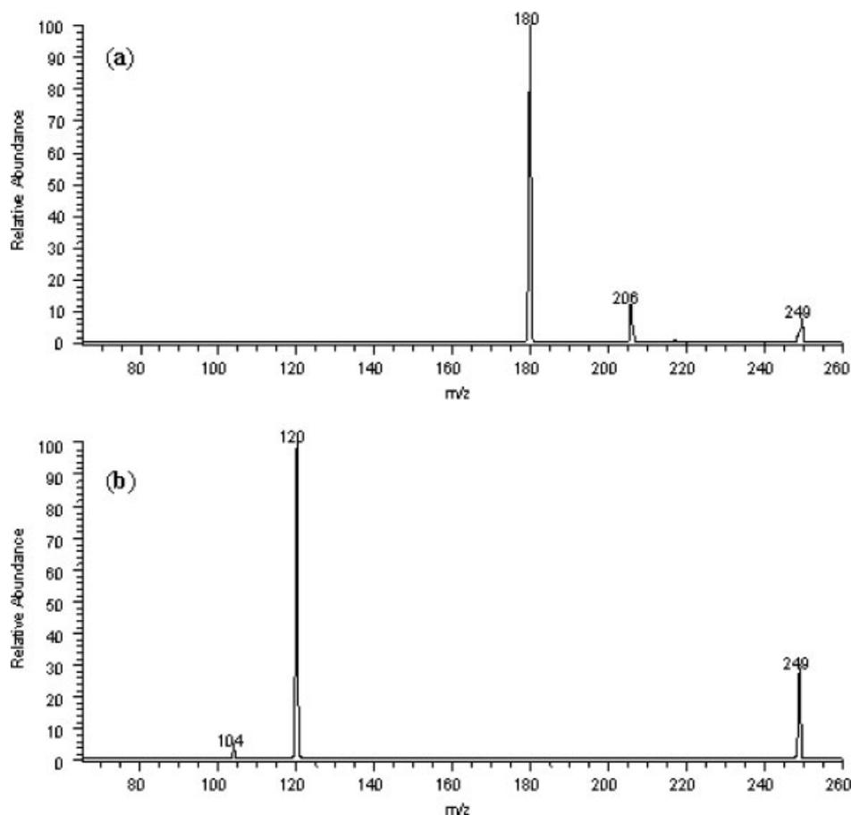
**Figure 2.** ESI-MS<sup>3</sup> spectra of  $m/z$  249 of (a) **1** and (b) **3** at 22 eV.
