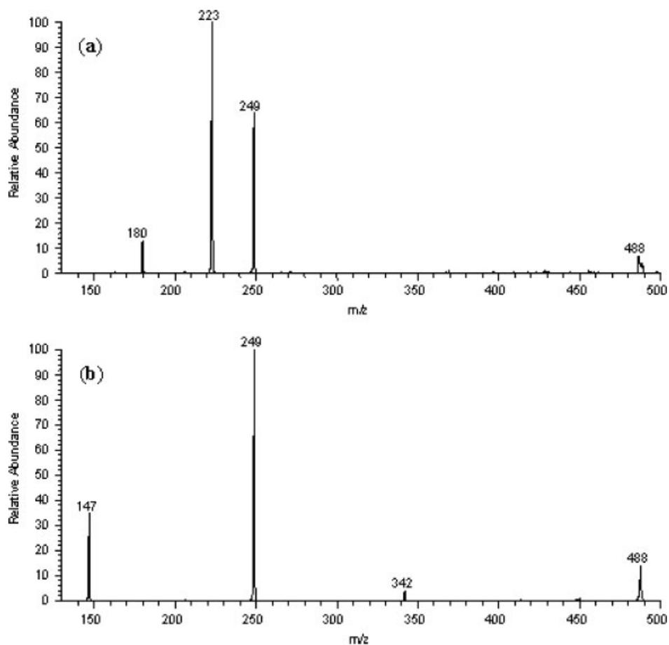
**Figure 1.** ESI-MS/MS spectra of  $[M + H]^+$  ions ( $m/z$  488) of (a) **1** and (b) **3** at 18 eV.
