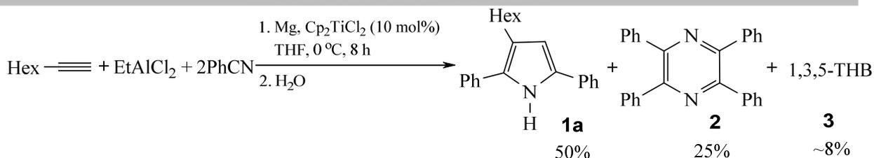
**Scheme 1.** Reaction of oct-1-yne with benzonitrile and  $\text{EtAlCl}_2$  catalyzed by  $\text{Cp}_2\text{TiCl}_2$  in tetrahydrofuran
