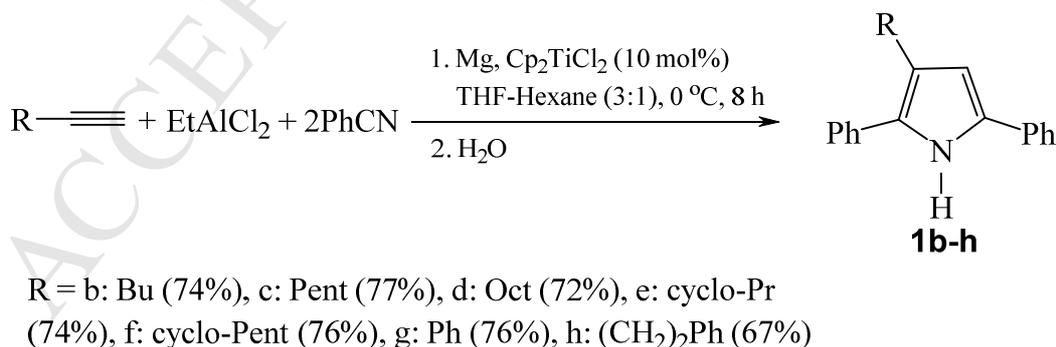
**Scheme 3.** Synthesis of 2,3,5-substituted 1*H*-pyrroles by the reaction of terminal acetylenes with benzonitrile and  $\text{EtAlCl}_2$  catalyzed by  $\text{Cp}_2\text{TiCl}_2$ .
