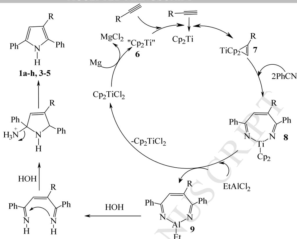
**Scheme 5.** Possible pathway for the formation of 2,3,5-substituted 1*H*-pyrroles from terminal acetylenes, nitriles and ethylaluminum dichloride in the presence of the  $\text{Cp}_2\text{TiCl}_2$  catalyst.
