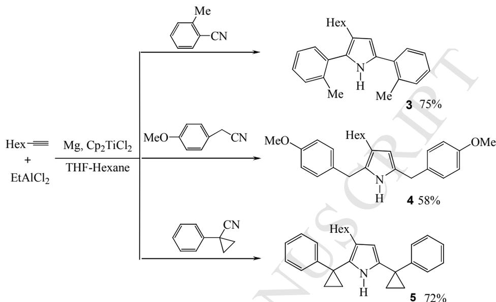
**Scheme 4.** Synthesis of 2,3,5-substituted 1*H*-pyrroles by the reaction of oct-1-yne with aromatic nitriles and EtAlCl<sub>2</sub> catalyzed by Cp<sub>2</sub>TiCl<sub>2</sub>.
