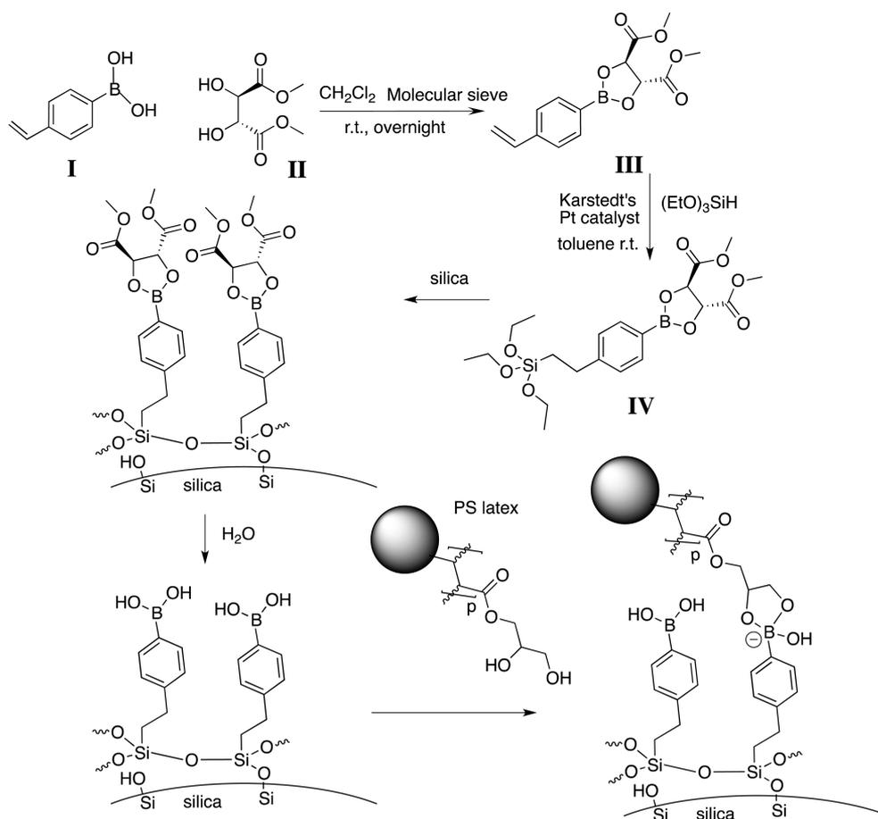
Poly(glycerol monomethacrylate)-stabilized polystyrene latex (PGMA-PS) was supplied by S. Armes (their designation KLT 156). Latex preparation and characterization was described previously.<sup>20</sup> The hydrodynamic diameter of the particle was of 177 nm, and the electrophoretic mobility was close to zero. The poly(glycerol monomethacrylate) stabilizer chains had a degree of polymerization of 50, and the stabilizer coverage was 3.2 mg m<sup>-2</sup>.
