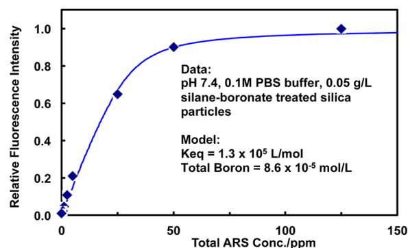
**Figure 3.** ARS binding to silaneboronate-treated silica. Theoretical curve was fit by varying the boronate–ARS binding constant. Incident wavelength was 468 nm, and fluorescence intensity was measured at 517 nm.
