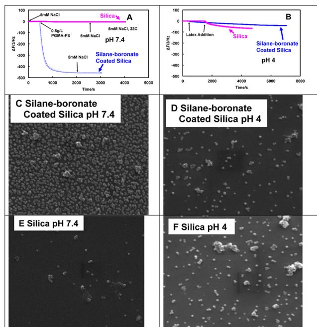
**Figure 2.** PGMA-PS deposition onto silica QCM-D sensors before and after silaneboronate treatment. SEMs micrographs show images of QCM-D sensor surfaces after the deposition experiment.
