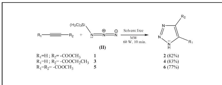
A fast one-pot microwave-assisted solvent free synthesis of simple alkyl 1,2,3-triazole-4-carboxylate derivatives by 1,3-dipolar cycloaddition reactions with trimethylsilyl azide ( $Me_3Si-N_3$ ) on the alkylpropiolates and DMAD in high yields is described.
