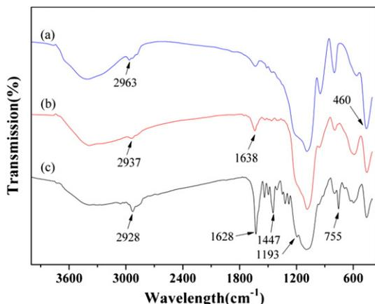
Fig. 1. FT-IR spectra of (a) SMNPs, (b) SMNPs-Salen and (c) SMNPs-Salen Pd (II).
