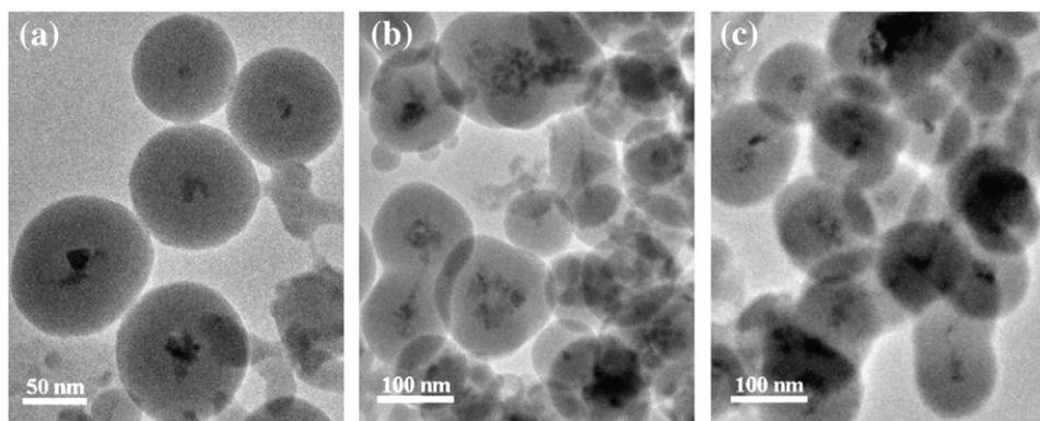
Fig. 2. TEM images of (a) SMNPs, (b) SMNPs-Salen Pd (II) and (c) SMNPs-Salen Pd (II) after the five cycles.
