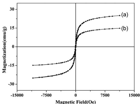
Fig. 4. Room temperature magnetization curve of (a) SMNPs and (b) SMNPs-Salen Pd (II).
