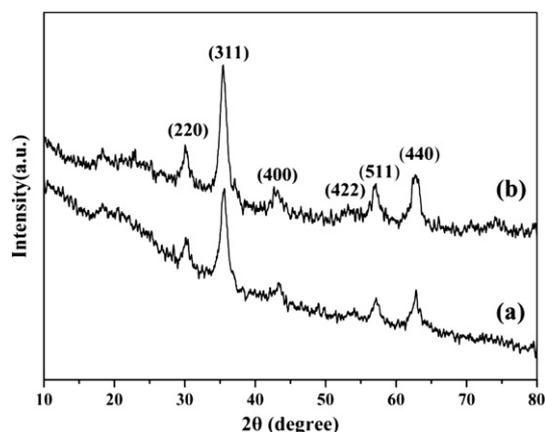
Fig. 3. XRD pattern of (a) SMNPs and (b) SMNPs-Salen Pd (II).
