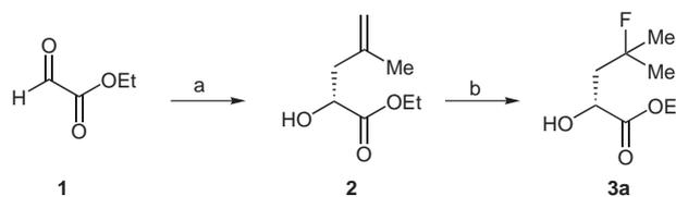
**Scheme 2** Reagents and conditions: (a)  $\text{TiCl}_2(\text{O}i\text{-Pr})_2$  (5 mol%, 0.3 M toluene), (*R*)-BINOL (7 mol%), isobutylene (4 equiv), 4 Å MS (2.9 g/g),  $\text{ZnCl}_2$  (5 mol%), toluene,  $-78^\circ\text{C}$  then  $4^\circ\text{C}$ , 16 h, Darco KB-B (1 g/g), heptane, 57%, >95% ee; (b) HF-pyridine (20 equiv), heptane,  $0^\circ\text{C}$ , 2 h, 71%, >95% ee.
