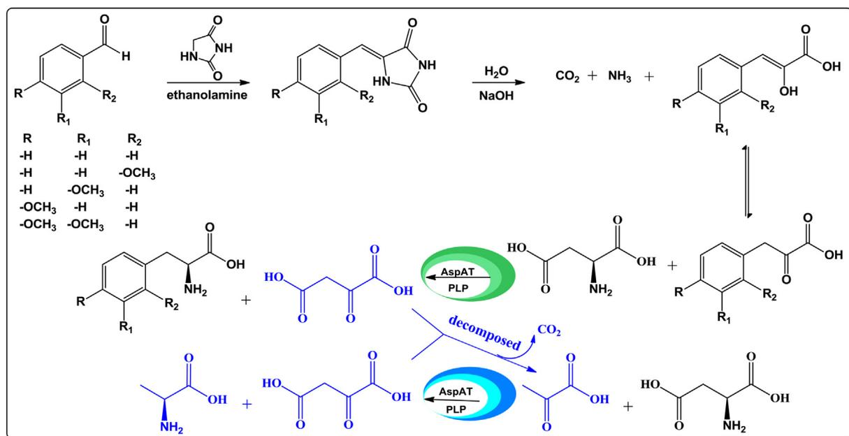
**Scheme 1.** Synthesis of L-DM-Phe and its analogues via the engineered or wild type AspAT. AspAT = aspartate aminotransferase from *Escherichia coli* K-12, PLP = pyridoxal phosphate.
