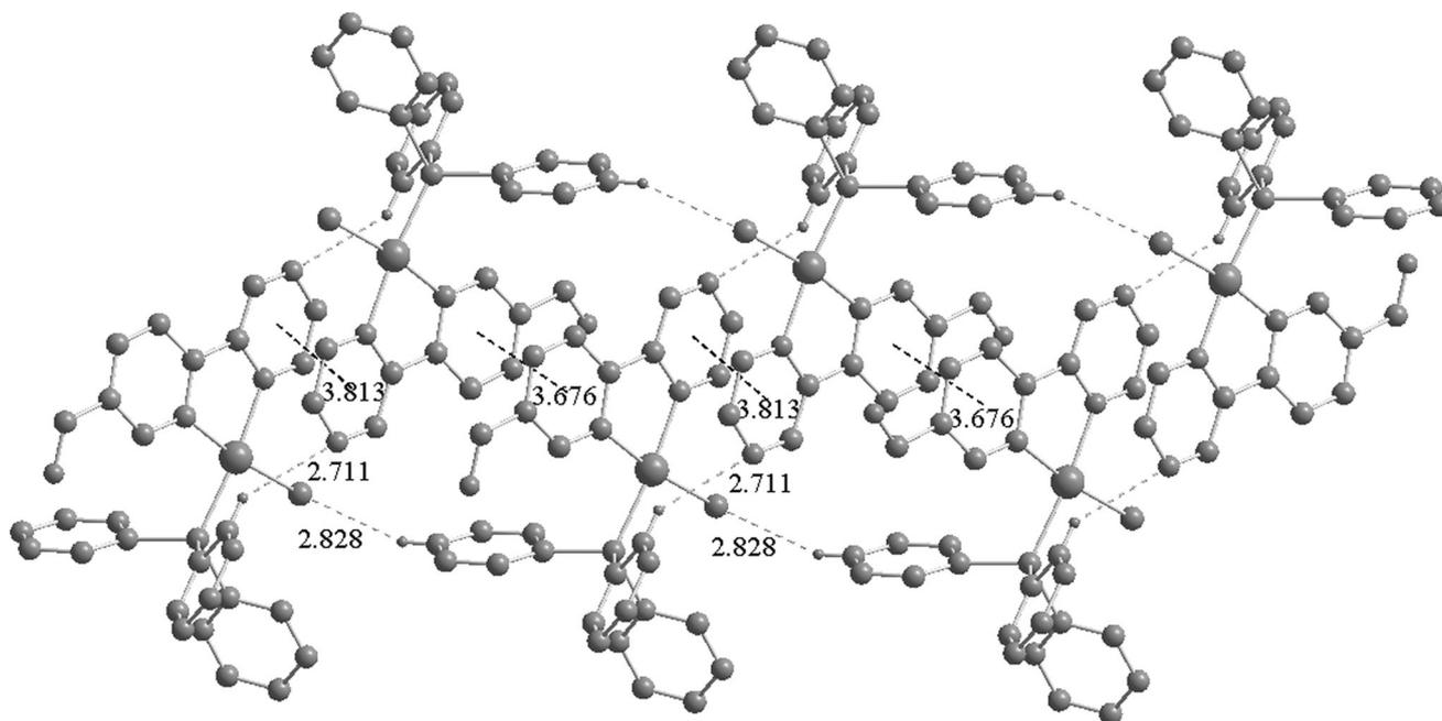
**Fig. 3** One-dimensional lamellar structure of complex **2** formed by C–H···Cl(N) hydrogen bonds and  $\pi$ – $\pi$  interactions. Non-hydrogen bonding H atoms are omitted for clarity
