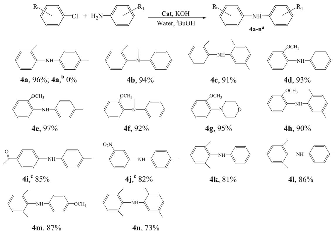
**Scheme 2** Amination of various aryl chlorides catalyzed by palladacycles. Reaction conditions: aryl chlorides (1.0 mmol), amine (1.2 mmol), **3** (0.5 mol %), KOH (3.0 mmol), *t*BuOH (4.0 mmol), H<sub>2</sub>O (3 mL), 100 °C, 12 h. <sup>a</sup>Isolated yield. <sup>b</sup>Catalyst **2** (0.5 mol %). <sup>c</sup>Catalyst **3** (0.2 mol %)
