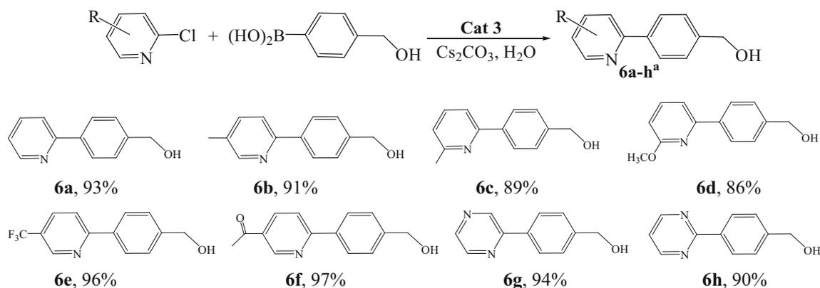
**Scheme 4** Coupling of *N*-heteroaryl chlorides with 4-(hydroxymethyl)phenylboronic acid catalyzed by **3**. Reaction conditions: *N*-heteroaryl chlorides (1.0 mmol), 4-HOCH<sub>2</sub>-PhB(OH)<sub>2</sub> (1.5 mmol), **3** (0.2 mol %), Cs<sub>2</sub>CO<sub>3</sub> (2.0 mmol), H<sub>2</sub>O (3 mL), 100 °C, 12 h. <sup>a</sup>Isolated yield
