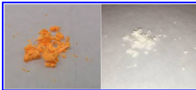
Figure 7. Digital photographs of bulk polymer material before (left) and after (right) the enzymatic reaction.
