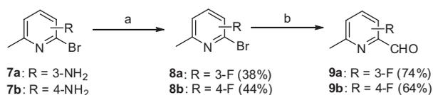
**Scheme 1.** Reagents and conditions: (a) (i) concn HCl, NaNO<sub>2</sub>, 0 °C, 10 min; (ii) 65% HPF<sub>6</sub> in H<sub>2</sub>O, 100 °C, 10 min; (b) *n*-BuLi (1.6 M in hexane), anhydrous DMF, toluene, –78 °C, 2 h.
