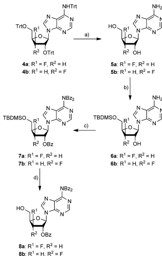
**Scheme 4.** a) TFA,  $\text{CH}_2\text{Cl}_2$ , RT, 1 h, **5a** (94%), **5b** (76%); b) TBDMSCl, DMAP, pyridine, RT, overnight, **6a** (36%), **6b** (22%); c) BzCl, pyridine, RT, overnight, **7a** (90%), **7b** (quant.); d) TFA/ $\text{H}_2\text{O}$  1:1, THF, RT, 1 h, **8a** (90%), **8b** (81%).
