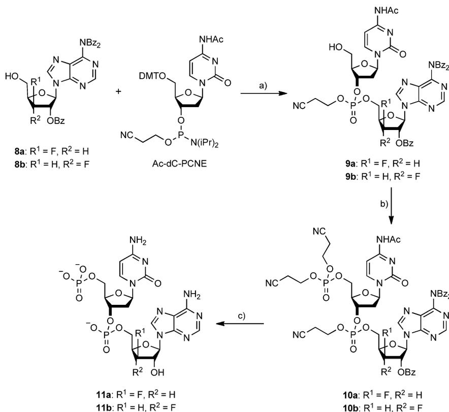
**Scheme 5.** a) i: Tetrazole, CH<sub>2</sub>Cl<sub>2</sub>, RT, 1 h; ii: I<sub>2</sub>, H<sub>2</sub>O/Pyr/THF, RT, 30 min; iii: TCA, CH<sub>2</sub>Cl<sub>2</sub>, RT, 30 min, **9a** (72%), **9b** (70%); b) i: bis(2-cyanoethyl)diisopropylphosphoramidite, tetrazole, CH<sub>2</sub>Cl<sub>2</sub>, RT, 1 h; ii: I<sub>2</sub>, H<sub>2</sub>O/Pyr/THF, RT, 30 min, **10a** (80%), **10b** (87%); c) CH<sub>3</sub>NH<sub>2</sub>, EtOH/H<sub>2</sub>O, RT, 24 h, **11a** (34%), **11b** (46%).
