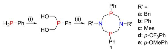
**Scheme 3.** Synthesis of  $P^R_2N^{R'}_2$  ligands used in this study. Conditions: (i)  $p$ - $CH_2O$ , EtOH, 78 °C, 4 h; (ii) dropwise  $H_2NR'$ , EtOH, 78 °C, 24 h. Yield **1c** = 15%; **1a-b**, **1d-e** are known.<sup>[5,7]</sup>
