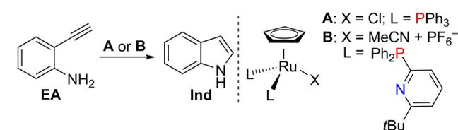
**Scheme 1.** Cyclization of 2-ethynylaniline (**EA**) with a) a non-cooperative catalyst **A** (10 mol% **A**, pyridine, 90 °C, 25 min, 84% **Ind**)<sup>[2e]</sup> and b) a cooperative catalyst **B** (2 mol% **B**, THF, 70 °C, 7 h, 87% **Ind**).<sup>[2f]</sup> [Please use corrected scheme 1 (cdx file attached) in which the structure of **A** is corrected]
