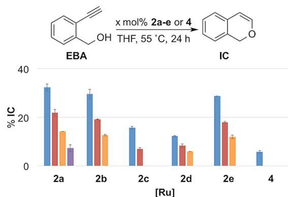
**Figure 4.** Cyclization yields of 2-ethynylbenzyl alcohol (**EBA**) to isochromene (**IC**) in THF at 55 °C after 24 h with catalysts **2a–e** and **4** at 3 mol% (blue), 1 mol% (red), 0.5 mol% (orange) and 0.1 mol% (purple).
