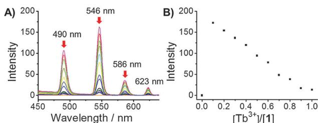
Fig. 1 (A) Photoluminescence spectra of supramolecular gel **1** (5 wt%) with various concentration of Tb<sup>3+</sup> (0–1.0 equiv.). (B) Plot of photoluminescence intensity against mole ratio of [Tb<sup>3+</sup>]/**1**.
