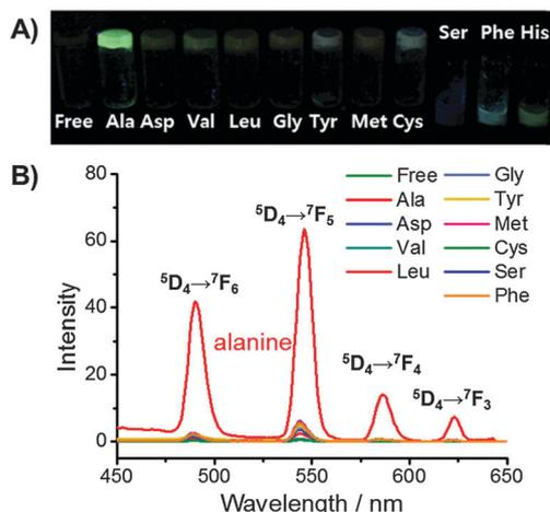
Fig. 3 (A) Photograph of supramolecular gel **1** (5 wt%) with Tb<sup>3+</sup> (1 equiv.) upon addition of amino acids (3 mM) under a UV lamp. (B) Photoluminescence spectra of supramolecular gel (5 wt%) with Tb<sup>3+</sup> (1 equiv.) upon addition of amino acids (3 mM).
