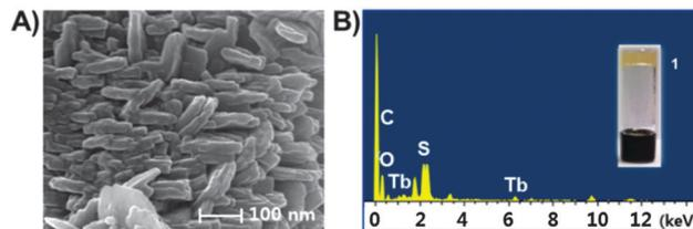
Fig. 2 (A) SEM image of xerogel **1** (5 wt%) with Tb<sup>3+</sup> (1 equiv.). (B) EDX spectrum of xerogel **1** with Tb<sup>3+</sup>.
