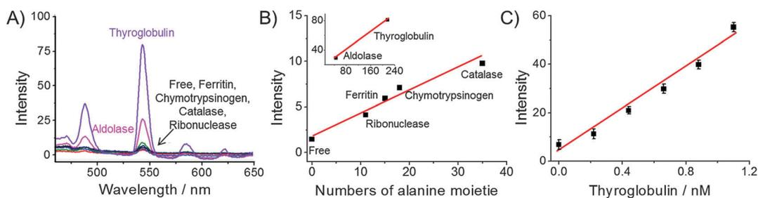
Fig. 4 (A) Photoluminescence spectra of supramolecular gel **1** (5 wt%) with Tb<sup>3+</sup> (1 equiv.) upon addition of various proteins containing alanine moiety; ferritin, aldolase, thyroglobulin, chymotrypsinogen, catalase and ribonuclease. (B) Plot of photoluminescence intensity of numbers of alanine moiety at 546 nm. (C) Plot of photoluminescence intensity of supramolecular gel with Tb<sup>3+</sup> upon addition of thyroglobulin (0.22–1.12 nM) at 546 nm.
