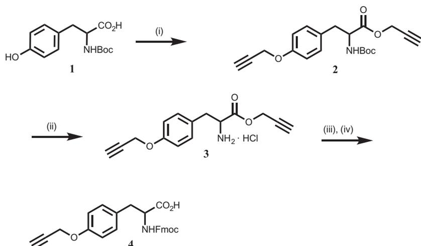
**Scheme 1.** Reagents and conditions: (i)  $K_2CO_3$ , propargyl bromide, DMF, 18 h, rt; (ii) AcCl, MeOH, 4 h, 0 °C to rt; (iii) NaOH, MeOH, 1.5 h, HCl,  $H_2O$ , 4 °C, 18 h; (iv)  $NaHCO_3$ , FmocOSu, dioxane,  $H_2O$ .
