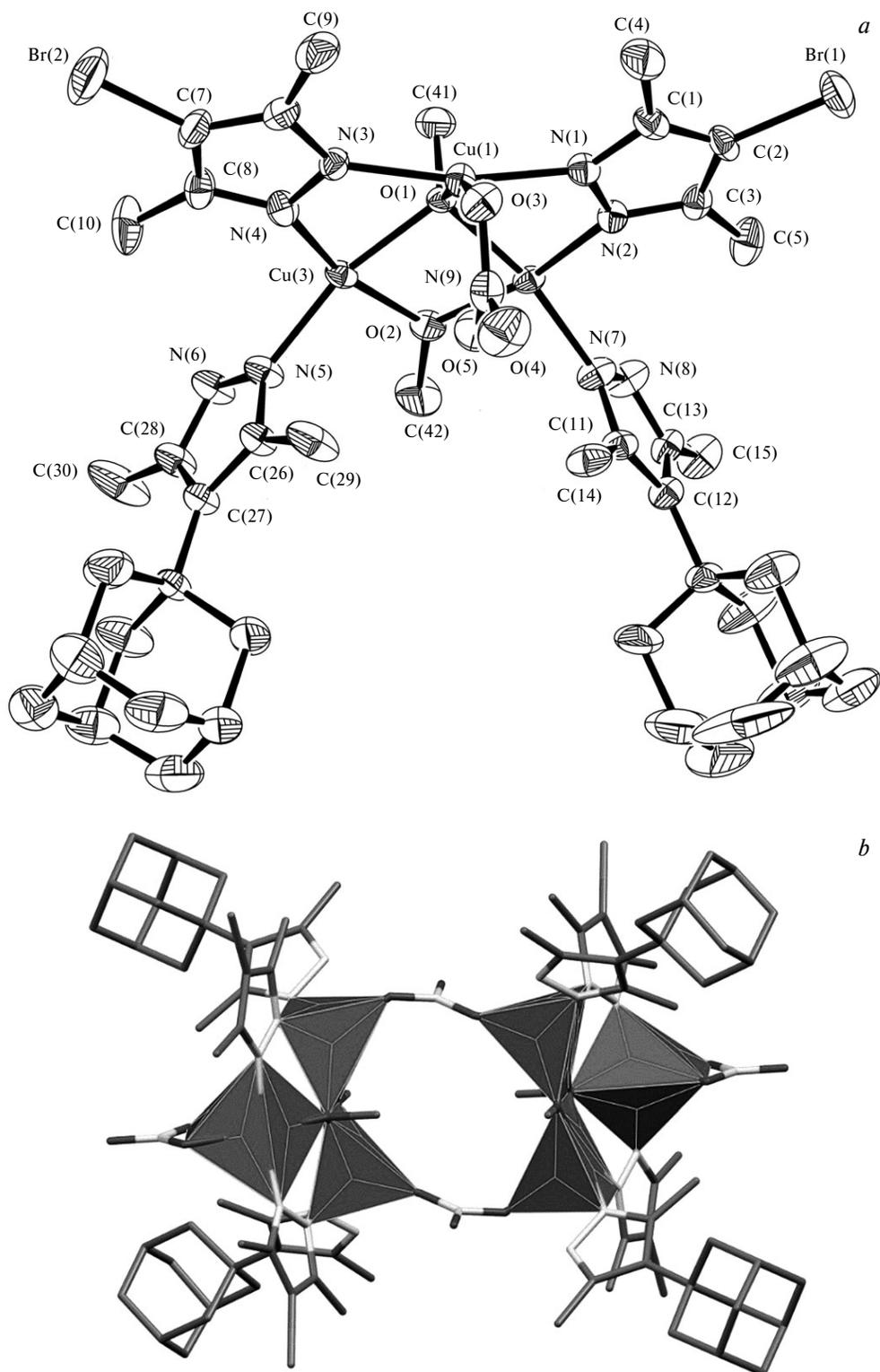
**Fig. 5.** Asymmetric unit of the crystal structure of compound 7 with thermal ellipsoids drawn at 50% probability level (*a*) and the molecular structure of hexanuclear complex 7 (*b*). Hydrogen atoms and the atom numbering of adamantane moieties are omitted for clarity.
