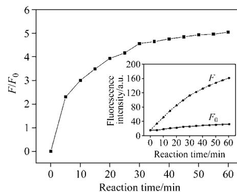
**Figure 3** Effect of reaction time on fluorescence intensity of 4-MUDNBS ( $4.0 \mu\text{mol}\cdot\text{L}^{-1}$ ) cleavage system by SNH ( $5.0 \mu\text{g}\cdot\text{mL}^{-1}$ ).  $F$  and  $F_0$  are the fluorescence intensity of 4-MUDNBS solution in the presence and absence of SNH, respectively. Other conditions were the same as those described in the experimental section.
