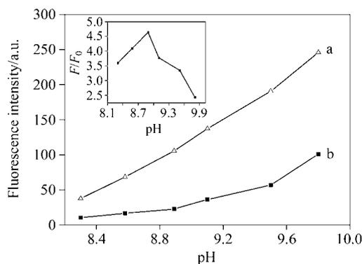
**Figure 4** Effect of pH on the fluorescence intensity of 4-MUDNBS ( $4.0 \mu\text{mol}\cdot\text{L}^{-1}$ ) in the presence (a) and absence (b) of SNH ( $5.0 \mu\text{g}\cdot\text{mL}^{-1}$ ) in pH  $\text{NH}_3\text{-NH}_4\text{Cl}$  buffer solution. Inset: fluorescence enhancement factor  $F/F_0$  as a function pH value.
