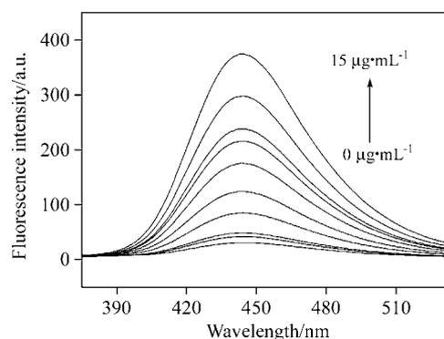
**Figure 1** Fluorescence emission spectra (excitation at 350 nm) of 4-MUDNBS ( $4.0 \mu\text{mol}\cdot\text{L}^{-1}$ ) toward different concentrations of SNH (final concentrations: 0, 0.5, 1.0, 3.0, 5.0, 7.0, 9.0, 10, 12, 15  $\mu\text{g}\cdot\text{mL}^{-1}$ ) after incubation at room temperature for 35 min in pH 8.9  $\text{NH}_3\text{-NH}_4\text{Cl}$  buffer.
