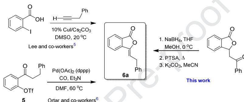
**Scheme 2.** Synthesis of 3-(2-phenylethylidene)isobenzofuran-1(3H)-one **6a**.
