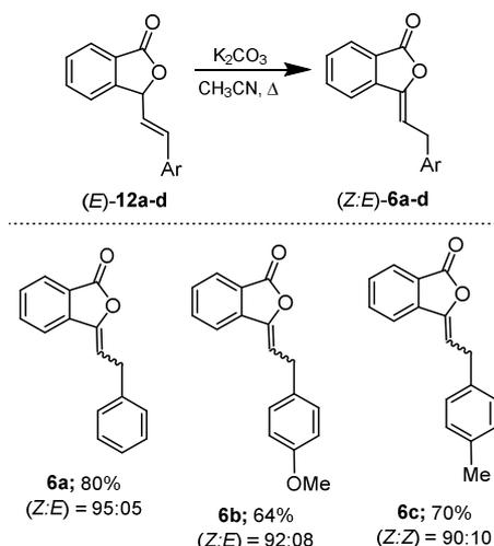
**Scheme 8.** Synthesis of 3-(2-arylethylidene)isobenzofuran-1(3H)-ones **6a-c**.
