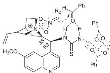
Fig. 2. Proposed reaction transition state.
