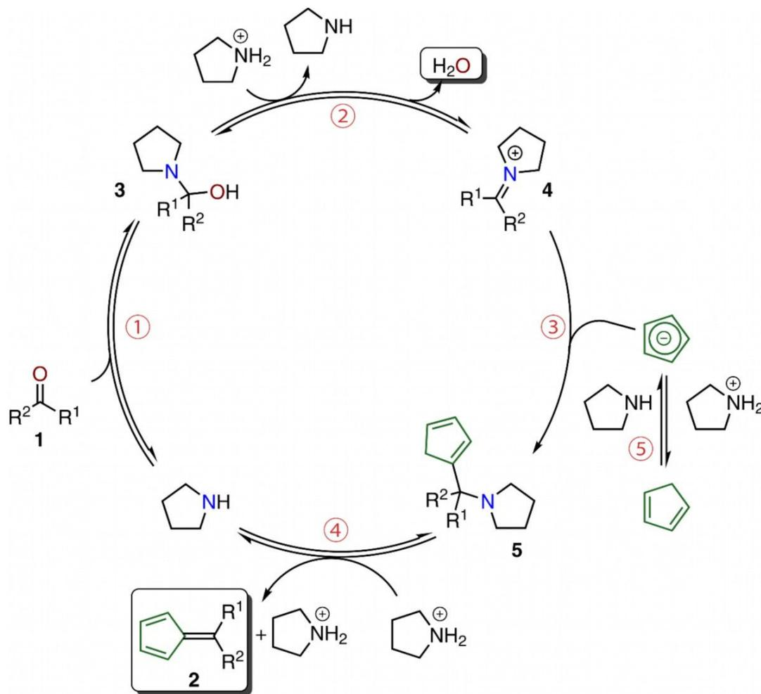
**Scheme 2** Catalytic cycle of the pyrrolidine-buffer catalyzed fulvene formation.
