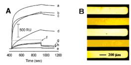
Figure 2. (A) SPR sensorgrams of SA adsorption on various mixed SAMs for  $\Gamma_{\rm I}$  = (a) 0.25, (b) 0.5, (c) 0.1, (d) 1.0, and (e) 0. Adsorption of SA (f) preblocked with excess free biotin at  $\Gamma_{\rm I} = 0.25$ . SPR sensorgrams for SAM surfaces for  $\Gamma_{\rm I}$  = (g) 0.5 and (h) 1.0 before electrochemical treatments. (B) Optical microscope image of pHRP-SA-patterned IDA.
