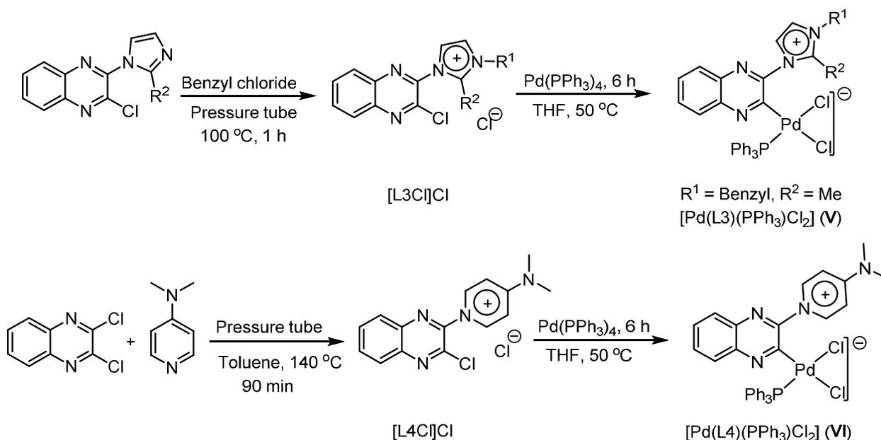
**Scheme 5** Synthesis of zwitterionic Pd(II) complexes **V** and **VI**
