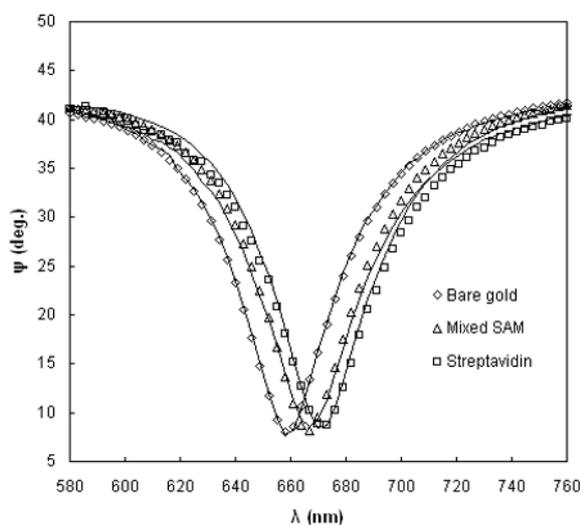
**Figure 2.** SPR ellipsometry spectra of parameter  $\psi$  for bare Au substrate; Au is coated with mixed compound **7**/compound **4** SAM; streptavidin is adsorbed onto the monolayer's surface (all spectra recorded in water). Experimental data points are shown with markers, smooth lines represent data fits.
