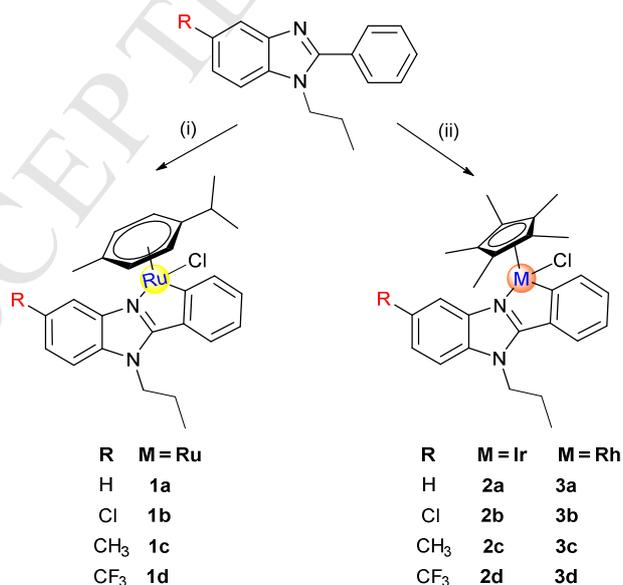
**Scheme 2** Transformation of 2-phenylbenzimidazoles to Ru, Ir and Rh cyclometallated complexes. Reagents and conditions: (i) [RuCl(*p*-cymene)]<sub>2</sub>/ NaOAc/ DCM/ rt; (ii) [RhCl(η<sup>5</sup>-C<sub>5</sub>H<sub>5</sub>)<sub>2</sub>] or [IrCl(η<sup>5</sup>-C<sub>5</sub>H<sub>5</sub>)<sub>2</sub>] / NaOAc/ DCM/ rt.
