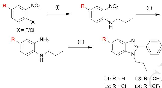
**Scheme 1** General synthetic approach to 2-phenylbenzimidazole ligands. Reagents and conditions: (i) *n*-PrNH<sub>2</sub>/ DMF/ rt; (ii) Zn/ NH<sub>4</sub>Cl/ MeOH/ rt; (iii) Benzaldehyde/ TFA/ MgSO<sub>4</sub>/ EtOH/ rt.
