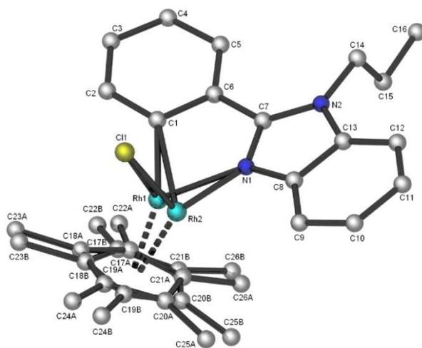
**Fig. 3** Molecular structure of complex **3a**, where thermal ellipsoids are drawn at 50% probability level.
