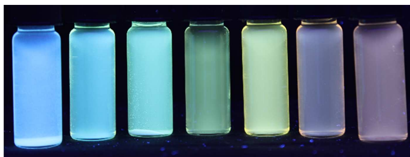
Figure 2. Fluorescence of 6p with variable solvent polarity (left to right: cyclohexane, toluene, ethyl acetate, dichloromethane, N,N -dimethyl formamide, acetonitrile; \lambda_{exc} = 365 nm, hand-held UV lamp).
