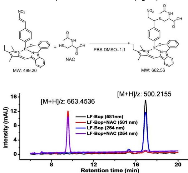
**Fig. 3.** HPLC and HRMS characterization of the thiol addition reaction on LF-Bop. LF-Bop (10  $\mu\text{M}$ ) was mixed with 400  $\mu\text{M}$  NAC in PBS (pH 7.4)/DMSO solution for 30 min before HPLC analysis. UV/VIS monitor was set at 254 nm and 581 nm.
