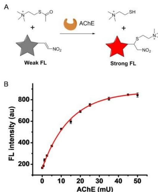
**Fig. 4.** A) Schematic show of the procedure to use LF-Bop for AChE activity evaluation; B) LF-Bop (10  $\mu\text{M}$ ) fluorescence turn on assay for monitoring AChE activity under different concentrations (0-50mU) in the presence of acetylthiocholine iodide (400  $\mu\text{M}$ ). The reaction was performed in PBS 7.4
