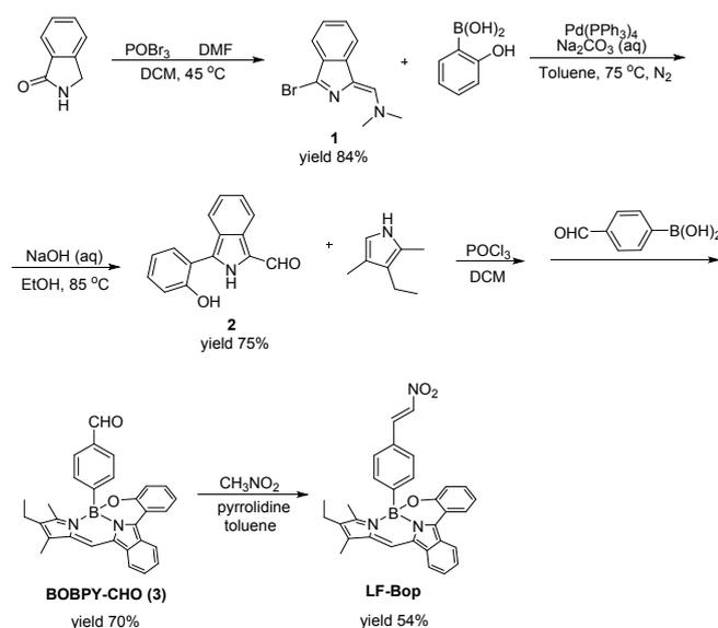
**Scheme 2.** Synthetic route of probe LF-Bop
