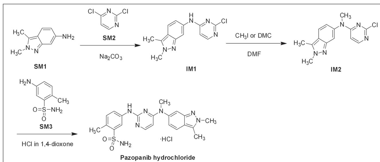
Scheme 1: Manufacturing process of pazopanib hydrochloride
