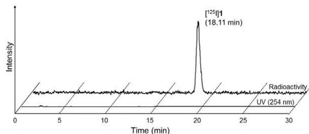
**Fig. 3.** HPLC analysis of [<sup>125</sup>I]**1**. HPLC conditions: the column was a COSMOSIL Cholesterol 4.6 mm × 250 mm, flow rate was 1.0 mL/min, UV excitation at 254 nm, mobile phase systems were CH<sub>3</sub>CN (0.1% TFA): H<sub>2</sub>O (0.1% TFA) = 60:40.
