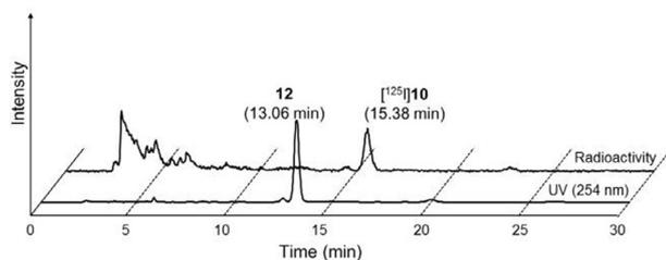
**Fig. 2.** HPLC analysis of [<sup>125</sup>I]**10** coinjected with precursor compound **12**. HPLC conditions: the column was a COSMOSIL Cholesterol 4.6 mm × 250 mm, flow rate was 1.0 mL/min, UV excitation at 254 nm, mobile phase systems were CH<sub>3</sub>CN (0.1% TFA): H<sub>2</sub>O (0.1% TFA) = 75:25.
