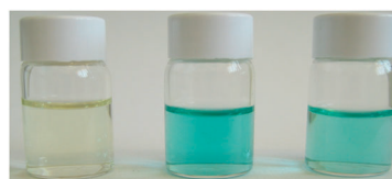
Fig. 2 Colour changes observed for probe 2 ( 1.0 \times 10^{-5} \text{ mol dm}^{-3} ) in acetonitrile upon addition of 100 equivalents of DCNP (middle) and 100 equivalents of DFP (right).
