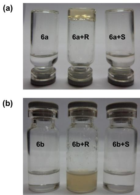
**Figure 1.** (a) photograph of the organogel formed by receptor **6a** ( $8.3 \times 10^{-3}$  M) in (10%) DMSO/ $\text{CHCl}_3$  with TBA salt of *R*-mandelic acid ( $8.5 \times 10^{-3}$  M); (b) photograph of the precipitate formed by receptor **6b** ( $9 \times 10^{-3}$  M) in (10%) DMSO/ $\text{CHCl}_3$  with TBA salt of *R*-mandelic acid ( $9 \times 10^{-3}$  M).
