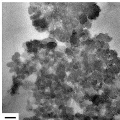
**Figure 3.** TEM image of the gel formed by receptor **6a** with TBA salt of *R*-mandelic acid; scale bar: 100 nm.
