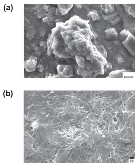
**Figure 2.** (a) SEM image of the gel formed by receptor **6a** with TBA salt of *R*-mandelic acid; scale bar:  $10\ \mu\text{m}$ . (b) SEM image of the precipitate formed by receptor **6b** with TBA salt of *R*-mandelic acid; scale bar:  $1\ \mu\text{m}$ .
