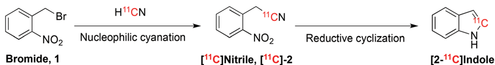
Scheme 2 Our design of synthesis [2- ^{11}\text{C} ]indole using [ ^{11}\text{C} ]HCN as radiolabeling precursor.
