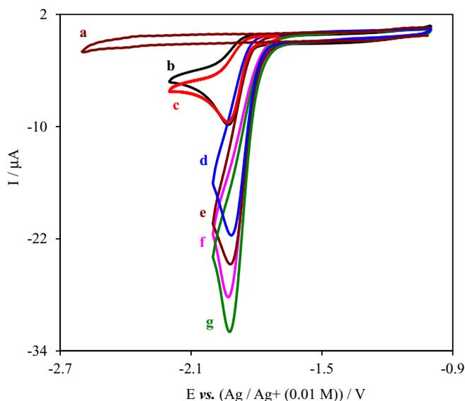
**Figure 1.** Cyclic voltammograms of a glassy carbon electrode in an acetonitrile solution containing 0.1 M TBAP and (a) 1.0 mM pyridine, (b) 1.0 mM NMPD, (c) 1.0 mM pyridine + 1.0 mM NMPD, (d) 1.0 mM NMPD in the presence of CO<sub>2</sub>. (e), (f) and (g) as (d) in the presence of 1.0, 2.0 and 3.0 mM pyridine respectively. Potential scan rate: 100 mV s<sup>-1</sup>.
