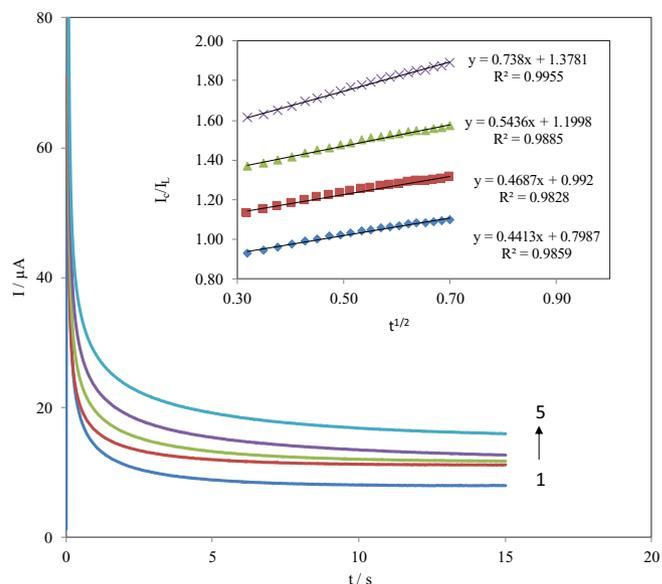
**Figure 2.** Chronoamperograms of a glassy carbon electrode in an acetonitrile solution containing 0.05 M TBAP, 1.0 mM NMPD and (a) saturated with CO<sub>2</sub>, (b), (c), (d) and (e) as (a) in the presence of 0.2, 0.3, 0.5, 0.7 mM pyridine, respectively. Inset shows plots of I<sub>C</sub>/I<sub>L</sub> vs. t<sup>1/2</sup> obtained from chronoamperograms 1–5.
