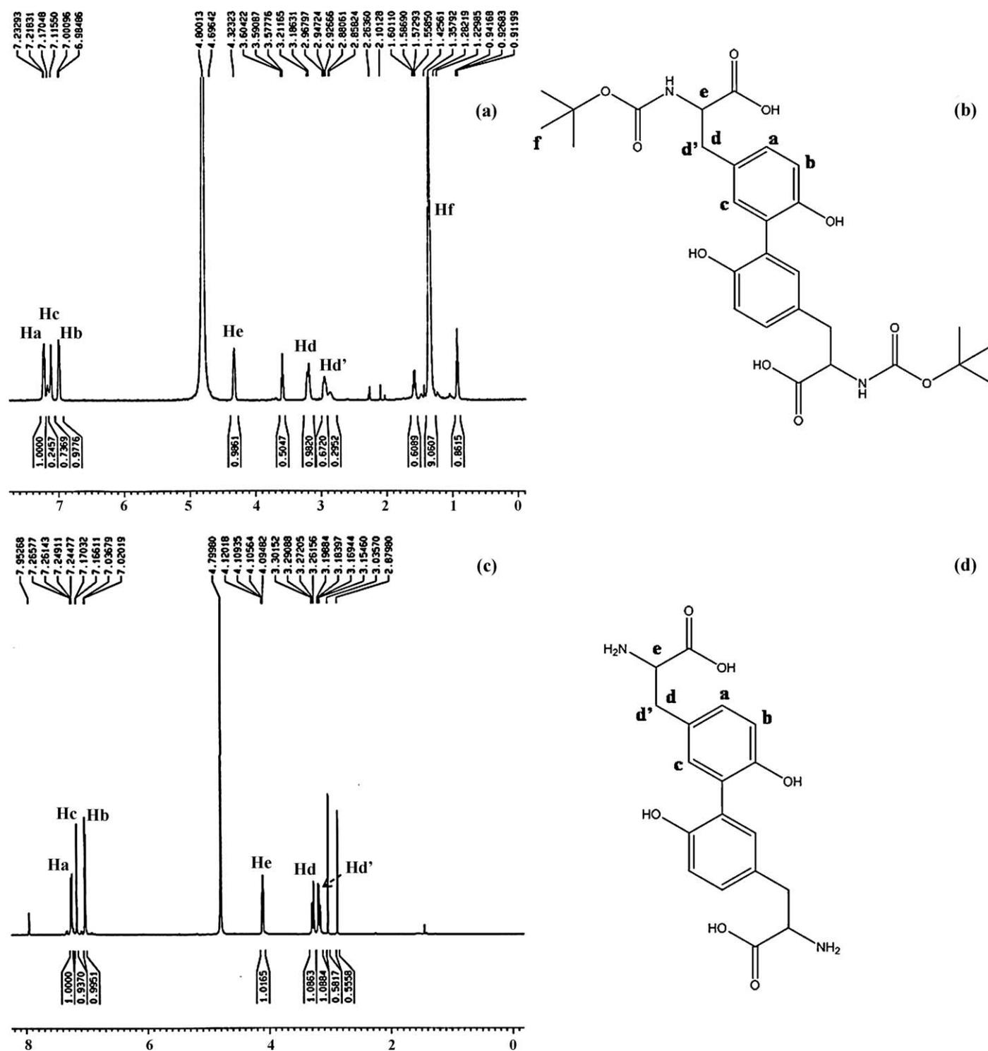
**Fig. 5.** <sup>1</sup>H NMR spectra of DBDY (A) and DY (C) obtained after the removal of Boc groups in DBDY. These spectra were recorded on a Bruker Avance 500-MHz nuclear magnetic resonance spectrometer (Bruker BioSpin Corp., Germany). Both compounds were dissolved in D<sub>2</sub>O. The chemical structures of DBDY and DY are shown in (B) and (D), respectively.
