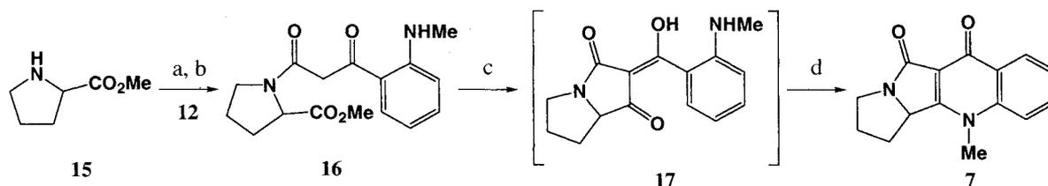
Conditions; (a) Et<sub>3</sub>N, CuI/THF, rt, 30 minutes; 77% (b) H<sub>2</sub>, Pd-C/EtOH, rt, 1 hour; 97% (c) NaOMe/MeOH, rt, 12 hours (d) AcOH, rt, 30 minutes; 84% in 2 steps
