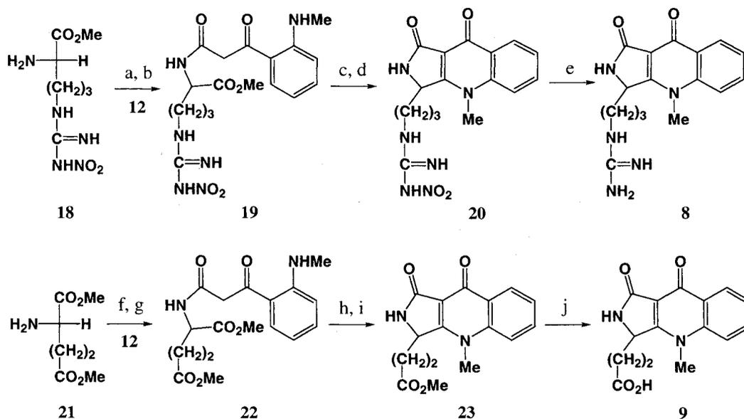
Conditions; (a) Et<sub>3</sub>N, CuI/THF, rt, 30 minutes; 78% (b) H<sub>2</sub>, Pd-C/EtOH, rt, 1 hour; 98% (c) NaOMe/MeOH, rt, 30 minutes (d) AcOH, rt, 30 minutes; 84% in 2 steps (e) H<sub>2</sub>, Pd(OH)<sub>2</sub>/10% AcOH-MeOH, rt, 30 minutes; 96% (f) Et<sub>3</sub>N, CuI/THF, rt, 30 minutes; 79% (g) H<sub>2</sub>, Pd-C/EtOH, rt, 1 hour; 93% (h) NaOMe/MeOH, 60°C, 4 hours (i) AcOH, 60°C, 5 minutes; 81% in 2 steps (j) NaOH/MeOH-H<sub>2</sub>O, 60°C, 1 hour; 83%
