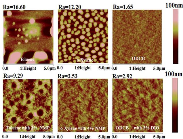
Fig. 4 AFM height images of PBBDTBT : PC<sub>71</sub>BM (1 : 1.5, w/w) blend films spin-coated from different solvents.
