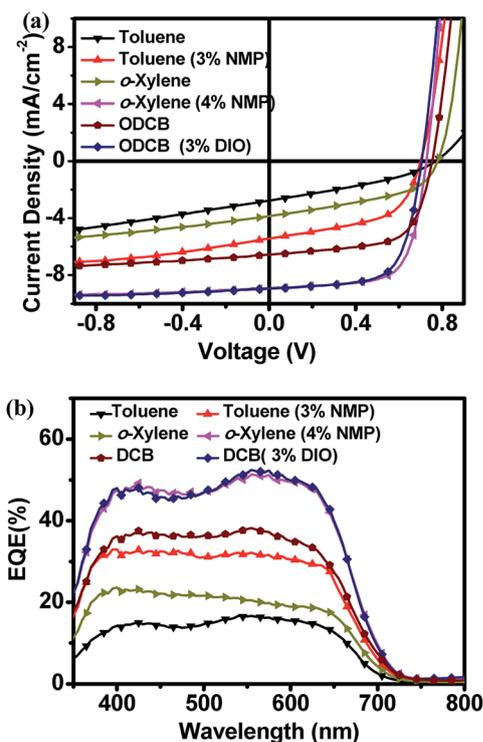
Fig. 3 (a) The  $J$ - $V$  characteristics of devices based on PBBDTBT : PC<sub>71</sub>BM under the illumination of AM1.5G ( $100 \text{ mW cm}^{-2}$ ); (b) EQE curves of solar cells fabricated under different conditions.
