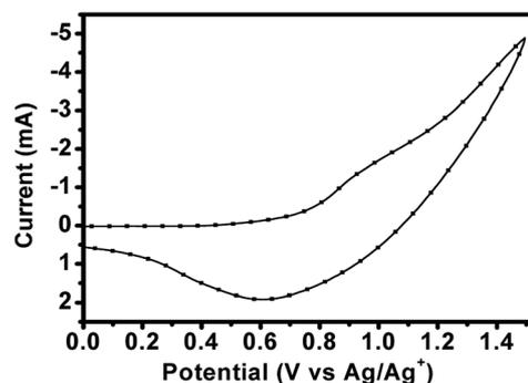
Fig. 2 Cyclic voltammogram of PBBDTBT as films on a platinum electrode in 0.1 mol L<sup>-1</sup> Bu<sub>4</sub>NPF<sub>6</sub> acetonitrile solution at a scan rate of 100 mV s<sup>-1</sup>.
