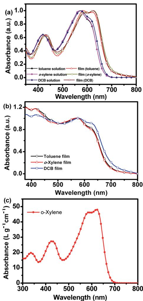
Fig. 1 UV-vis absorption spectra of (a) PBBDTBT in diluted toluene, *o*-xylene and DCB solutions and as films; (b) PBBDTBT : PC<sub>71</sub>BM (1 : 1.5 by weight) blending films spin coated from toluene, *o*-xylene and DCB solutions; (c) molar extinction coefficient of PBBDTBT in diluted *o*-xylene.
