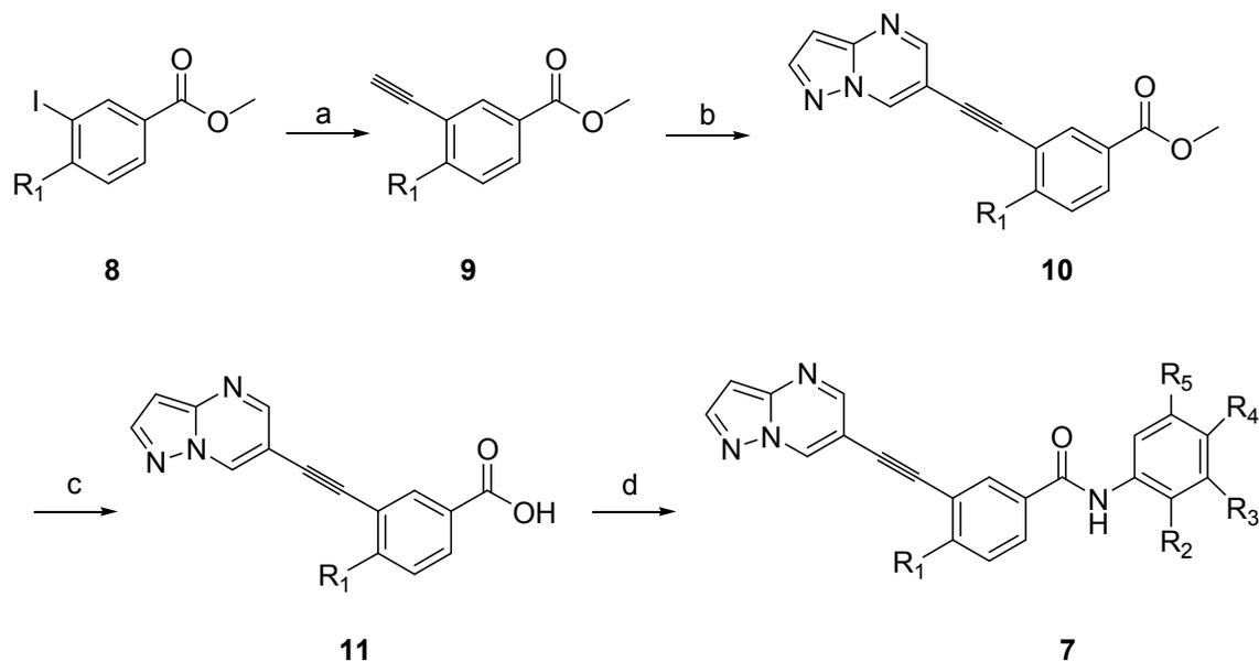
**Reagents and conditions:** (a) i) trimethylsilyl acetylene, CuI, PdCl<sub>2</sub>(PPh<sub>3</sub>)<sub>2</sub>, TEA, EtOAc, overnight, ~85.0%; ii) K<sub>2</sub>CO<sub>3</sub>, MeOH, 5 mins, 90.0-92.0%%; (b) CuI, PdCl<sub>2</sub>(PPh<sub>3</sub>)<sub>2</sub>, NMP, 80 °C, overnight, 80.0-85.0%; (c) NaOH, CH<sub>3</sub>OH, H<sub>2</sub>O, 50°C, 6 hrs, ~90.0%; (d) PyBOP, DIPEA, DCM, overnight, 40.0-90.0%.
