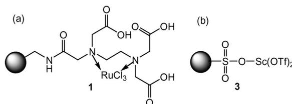
Figure 2. Illustration of the two immobilized Lewis acid catalysts investigated within the borosilicate glass micro reactor (a). Polymer-supported (ethylenediaminetetraacetic acid)ruthenium(III) chloride (PS-RuCl<sub>3</sub>) (**1**) and (b). Polymer-bound scandium(III) bis(trifluoromethanesulfonate) [PS-Sc(OTf)<sub>2</sub>] (**3**).
