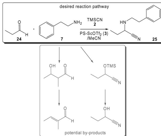
Scheme 2. Schematic illustrating a selection of the reaction products encountered when attempting to synthesize 2-(phenethylamino)butyronitrile (**25**) in a one-pot, batch reaction.
