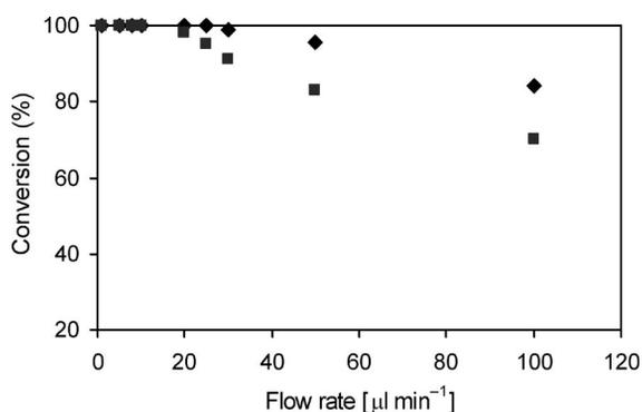
Figure 6. Illustration of the effect of flow rate on the synthesis of (◆) (*E*)-[1-(4-bromophenyl)methylidene]phenethyl-amine (**11**) and (■) 2-(4-bromophenyl)-2-(phenethylamino)acetonitrile (**8**) in a micro reactor.
