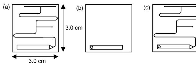
Figure 3. Schematic illustrating the components of the borosilicate glass reactor employed for the investigations described herein (a) top plate, (b) base plate and (c) bonded reactor.
