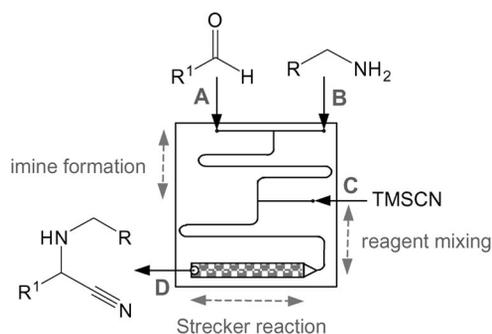
Figure 1. Diagrammatic representation of the reaction manifold used to evaluate the Strecker reaction conducted under continuous flow.
