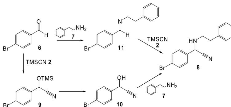
Scheme 1. Illustration of the model reaction selected for evaluation under continuous flow, depicting some of the possible by-products obtained and the reaction pathways followed in a one-pot transformation.
