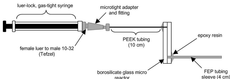
Figure 4. Schematic illustrating the technique employed for the connection of the micro reactor to a syringe driver.
