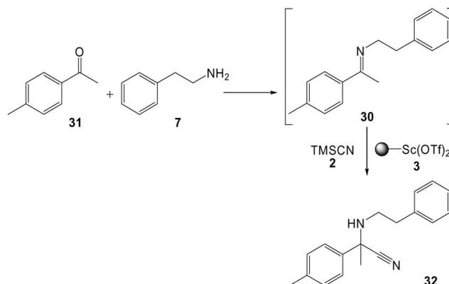
Scheme 3. Synthesis of 2-(phenylethylamino)-2-*p*-tolylpropanenitrile (**32**) investigated within a micro reactor.
