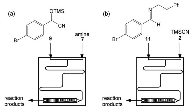
Figure 5. Reaction manifolds used to evaluate the order of addition for the synthesis of α-aminonitriles, catalyzed by PS-RuCl<sub>3</sub> (**1**), under continuous flow via (a) the *O*-TMS cyanohydrin **9** and (b) the imine **11**.
