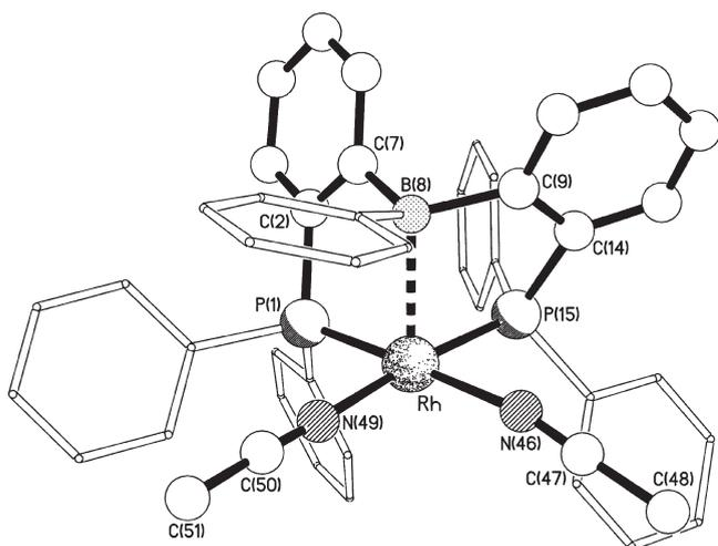
**Figure 3.** Molecular structure of  $[\text{Rh}(\text{MeCN})_2(\text{BPP})]^+$ . Selected bond lengths (Å) and angles (deg): Rh–P(1), 2.2298(7), Rh–P(15), 2.2631(7), Rh···B(8), 2.288(3), Rh–N(46), 2.104(3), Rh–N(49), 2.099(3), P(1)–Rh–B(8), 84.02(9), P(1)–Rh–P(15), 93.50(3), B(8)–Rh–P(15), 80.36(9), N(46)–Rh–N(49), 87.07(11).
