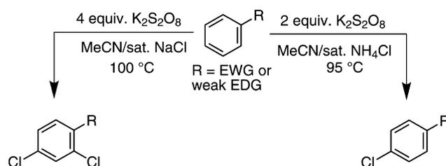
**Scheme 1.** Efficient combined systems for the chlorination of aromatic compounds.
