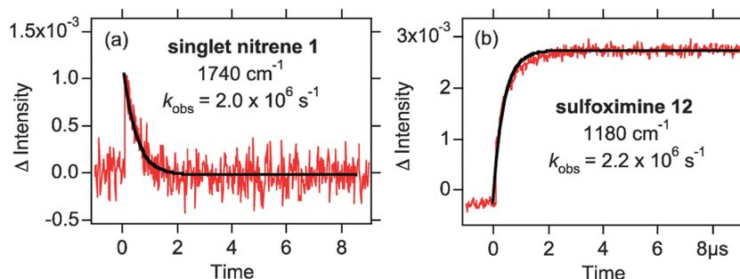
**Fig. 9** Kinetic traces observed at (a) 1740 and (b) 1180  $\text{cm}^{-1}$  following 266 nm laser photolysis of thiaziazole **2** (2 mM) in the presence of DMSO (5.3 M) in argon-saturated acetonitrile. The red curves are experimental data; the black curves are best fits to a single-exponential function. The error in derived rates is estimated to be  $\pm 10\%$ .
