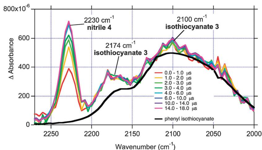
**Fig. 4** TRIR difference spectra averaged over the timescales indicated following 266 nm laser photolysis of thiazotriazole **2** (2 mM) in argon-saturated dichloromethane. Overlaid on the TRIR spectra is the normalized IR spectrum of phenyl isothiocyanate taken of an authentic sample under the same experimental conditions (black trace).
