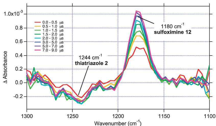
**Fig. 8** TRIR difference spectra averaged over the timescales indicated following 266 nm laser photolysis of thiaziazole **2** (2 mM) in argon-saturated acetonitrile.
