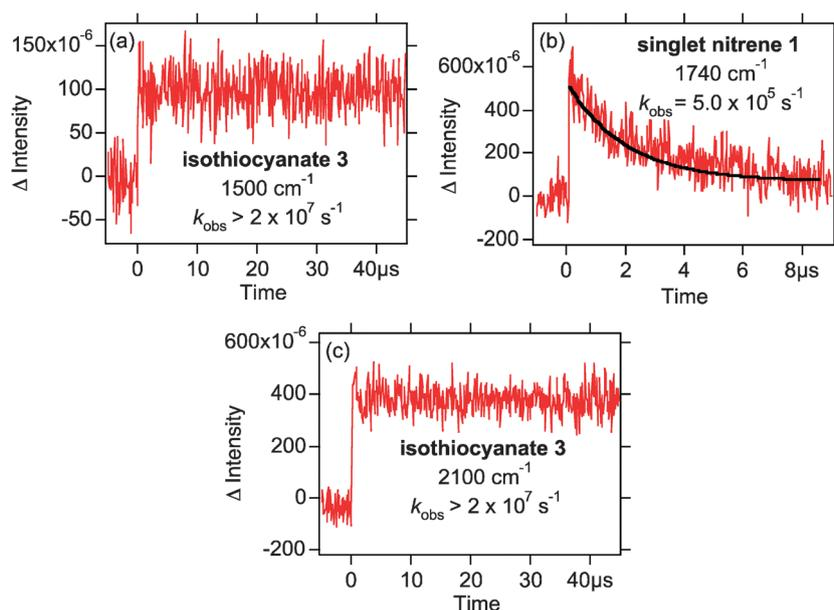
**Fig. 3** Kinetic traces observed at (a) 1500, (b) 1740, and (c) 2100  $\text{cm}^{-1}$  following 266 nm laser photolysis of thiazotriazole **2** (2 mM) in argon-saturated acetonitrile- $d_3$ . The red curves are experimental data; the black curve is the best fit to a single-exponential function. The error in derived rates is estimated to be  $\pm 10\%$ .
