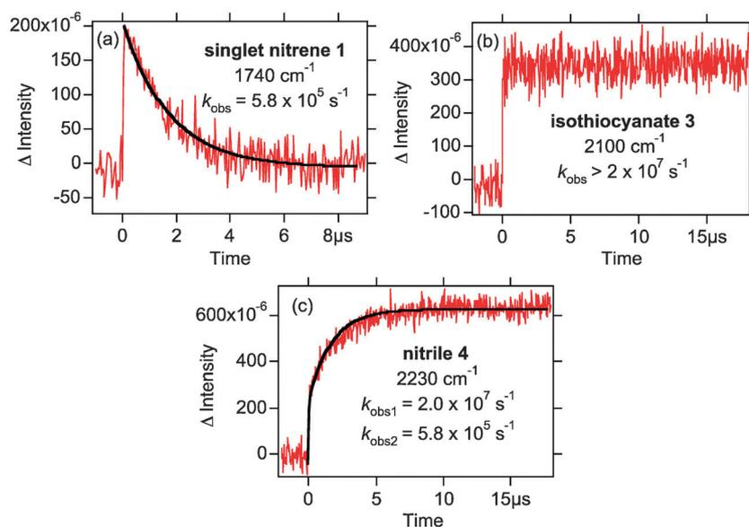
**Fig. 5** Kinetic traces observed at (a) 1740, (b) 2100, and (c) 2230  $\text{cm}^{-1}$  following 266 nm laser photolysis of thiazirazole **2** (2 mM) in argon-saturated dichloromethane. The red curves are experimental data; the black curves are best fits to a single- (a) or double- (c) exponential function. The error in derived rates is estimated to be  $\pm 10\%$ .
