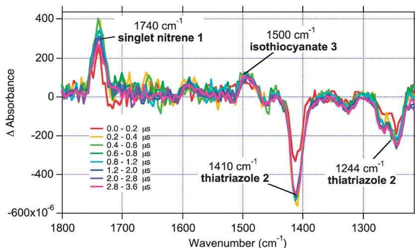
**Fig. 2** TRIR difference spectra averaged over the timescales indicated following 266 nm laser photolysis of thiazirazole **2** (2 mM) in argon-saturated acetonitrile- $d_3$ .
