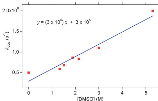
**Fig. 10** Plot of the observed rate of nitrene decay ( $k_{\text{obs}}$ ) monitored at 1740  $\text{cm}^{-1}$  versus the concentration of DMSO in acetonitrile ( $R^2 = 0.97$ ).
