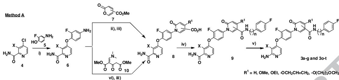
**Scheme 1.** Reagent and conditions: i) *t*-BuOK, DMF, 50°C for 6h, 76-82%; ii) DMAP, Molecular sieves, MeOH, 60°C for 2h, 81-85%; iii) NaOH, MeOH, H<sub>2</sub>O, 50°C for 2h, 86-92%; iv) BtOH, EDCI, DMAP, DCM, 25°C for 12h, 54-85%; v) PhI(OAc)<sub>2</sub>, EA, DCM, H<sub>2</sub>O, 0°C for 2h, 65-83%; vi) EtOH, 70°C for 2h, 86-90%.
