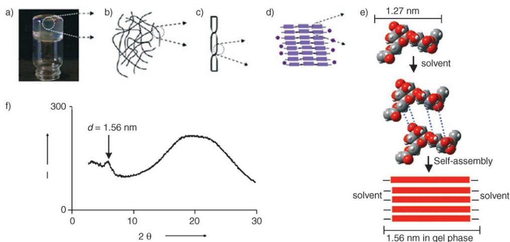
**Figure 2.** Proposed scheme of molecular packing. a) Gel formed by **1** in ethyl acetate, b) 3D network, c) fibers, d) multilayers, and e) modeled molecular packing. f) SAXS data for ethyl acetate gel of **1**.
