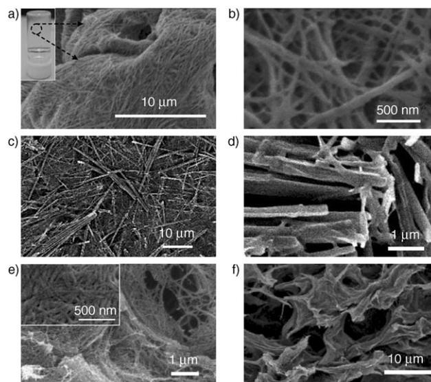
**Figure 1.** FE-SEM images of the organogels from a) **1** in ethyl acetate, b) **1** in ethyl acetate at a higher magnification, c) **1** in isopropanol, d) **1** in isopropanol at a higher magnification, e) **6** in ethyl acetate; inset shows higher magnification of **6** in ethyl acetate, f) **6** self-supporting and porous scaffold after UV polymerization in ethyl acetate.
