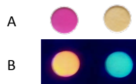
Figure 2. Sensing polyethylene oxide membranes containing probe 2 . A) Colour modulation of the sensing film in absence (left) and presence (right) of NO 2 (1 ppm) in air. B) Emission of the sensing film (excitation at 254 nm) in absence (left) and presence (right) of NO 2 (1 ppm) in air.
