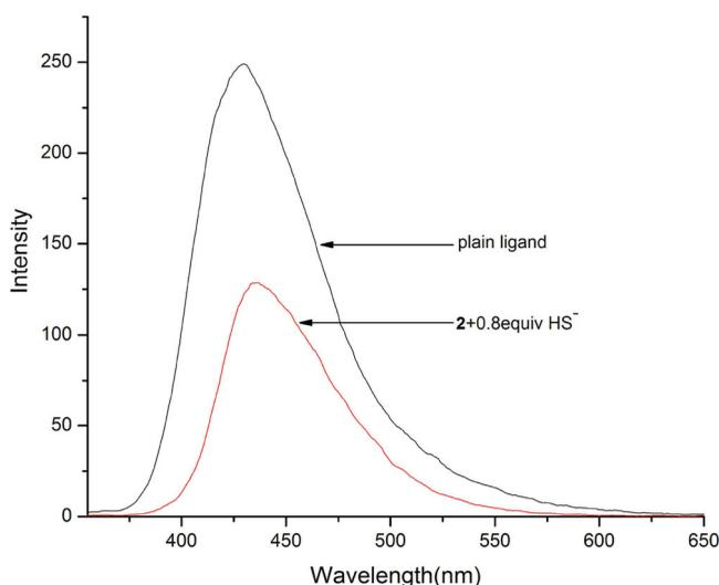
**Figure 7.** A comparison of fluorescence spectra of compounds **2** ( $4.0 \times 10^{-5} \text{ mol L}^{-1}$ ) in the presence of 0.8 equiv  $\text{HS}^-$  with the spectra of plain ligand ( $4.0 \times 10^{-5} \text{ mol L}^{-1}$ ).
