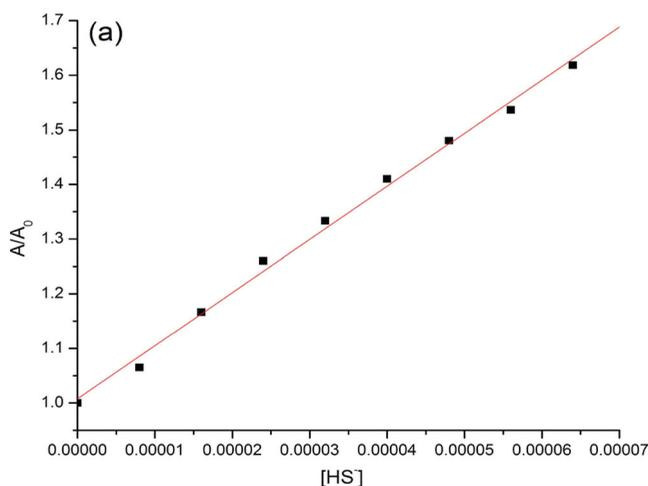
**Figure 4.** UV-VIS intensity of compound **1** in pour DMSO solution as a function of concentrations of  $\text{HS}^-$ .
