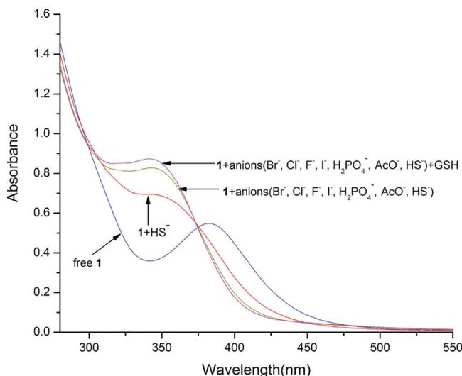
**Figure 3.** UV-vis spectral responses of compound **1** ( $4.0 \times 10^{-5} \text{ mol L}^{-1}$ ) upon the addition of 8 equiv anions ( $\text{AcO}^-$ ,  $\text{H}_2\text{PO}_4^-$ ,  $\text{F}^-$ ,  $\text{Cl}^-$ ,  $\text{Br}^-$  and  $\text{I}^-$ ) and 8 equiv GSH.
