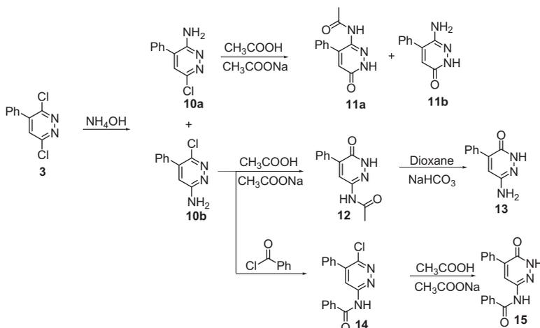
**Scheme 3a.** Synthesis of pyridazinone substituted amide **11–15**.
