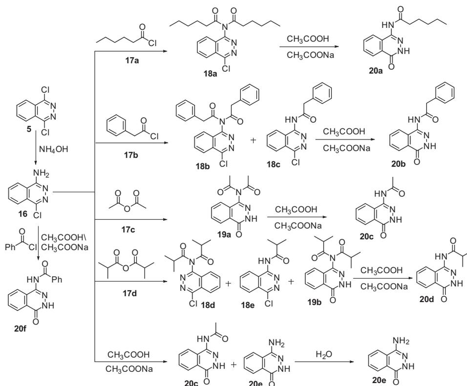
Scheme 3b. Synthesis of phthalazinone substituted amide **20a-f**.Table 1
