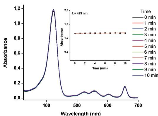
Figure 6. Photobleaching study for compound **11a** in  $\text{CH}_2\text{Cl}_2$  using a red laser (50 mW) at 661 nm.
