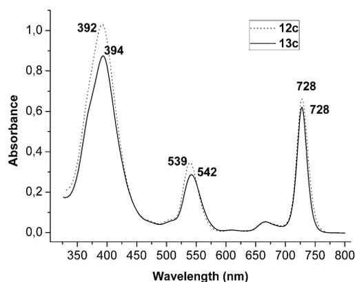
Figure 4. UV/Vis spectra of compounds **12c** and **13c** in  $\text{CH}_2\text{Cl}_2$ .
