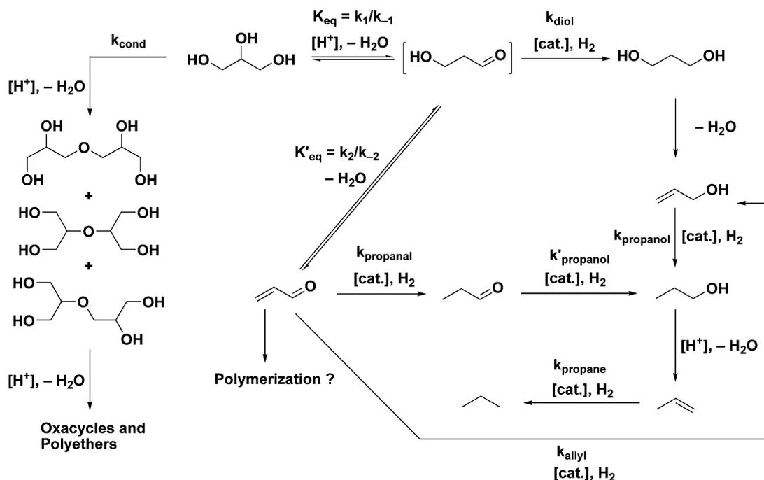
**Scheme 1** Conceivable pathways for the deoxygenation of glycerol catalyzed by a homogeneous Brønsted acid/metal complex based system.
