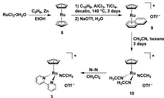
**Scheme 3** Preparation of  $[\text{cpRu}(\text{NCCH}_3)(\text{bipy})](\text{OTf})$ .
