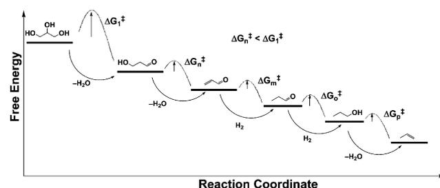
**Fig. 5** Reaction profile for the catalytic deoxygenation of glycerol under homogeneous Brønsted acidic conditions.
