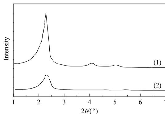
Fig. 1. XRD patterns of calcined Al-MCM-41 (1) and  $\text{VO}^{2+}/\text{MCM-41}$  (2).
