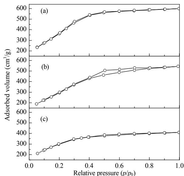
Fig. 2. Nitrogen adsorption-desorption isotherms of Al-MCM-41 (a),  $\text{VO}^{2+}/\text{Al-MCM-41}$  (b), and  $\text{VO}^{2+}/\text{Al-MCM-41}$  after the reaction (c).
